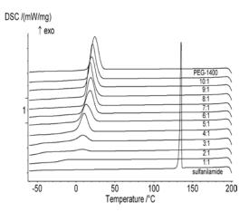
Fig. 6: DSC curves of initial samples of PEG-1400, sulfanilamide and their mixtures of varying composition (1-10:1) in dynamic atmosphere of argon 150 ml/min, in the temperature range of -60 to 200 °C (cooling). Cooling rate 10 °C/min.
