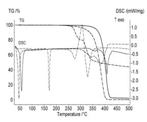
Fig. 1: TG/DSC curves of PEG-1000 (dashed line), PEG-1400 (solid lines) and sulfanilamide (dash and dot line) in dynamic atmosphere of argon 75 ml/min), in the temperature range 30 to 500 °C. Heating rate 5 °C/min.
