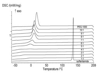
Fig. 3: DSC curves of initial samples of PEG-1000, sulfanilamide and their mixtures of varying composition (1-10:1) in dynamic atmosphere of argon 150 ml/min, in the temperature range of -60 to 200 °C (cooling). Cooling rate 10 °C/min
