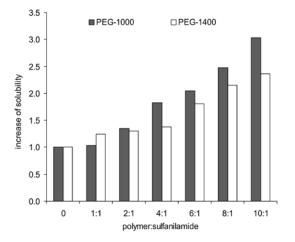
Fig. 8: Results of UV spectrophotometric analysis of water solutions of PEG-1000, PEG-1400 and sulfanilamide at various ratios of components. Optical density is taken at wavelength 261 nm.
