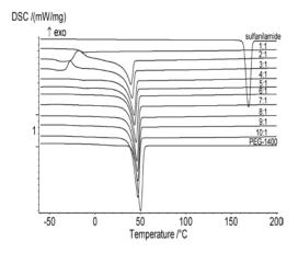
Fig. 7: DSC curves of initial samples of PEG-1400, sulfanilamide and their mixtures of varying composition (1-10:1) in dynamic atmosphere of argon 150 ml/min, in the temperature range of -60 to 200 °C (second heating). Heating rate 5 °C/min.
