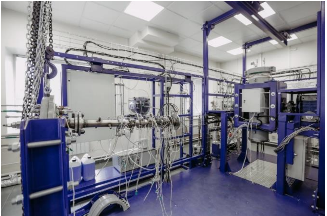
Fig. 22. Photo of a unique scientific installation for conducting physical modeling of the in-situ combustion process.
