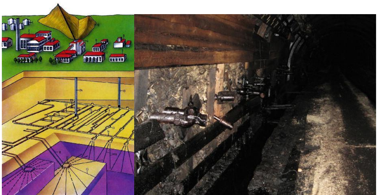
Fig. 8. Method for thermoshaft oil production.
