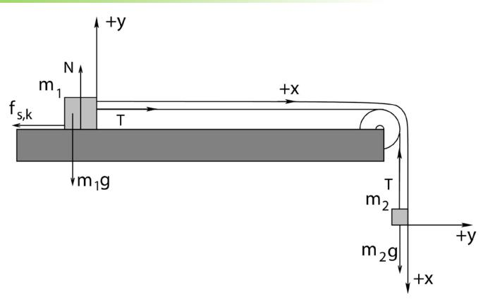
Atwood's machine, sort of, with one block resting on a table with friction and the other dangling over the side being pulled down by gravity near the Earth's surface. Note that we should use an "around the corner" coordinate system as shown, since a1 = a2 = a if the string is unstretchable.
