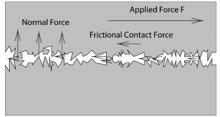
*Static Friction* is the force exerted by one surface on another that acts *parallel* to the surfaces to *prevent the two surfaces from sliding*.
