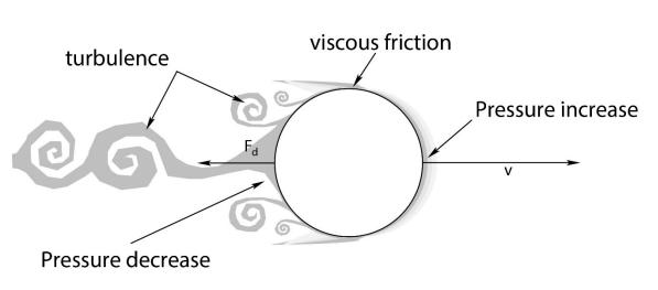
A "cartoon" illustrating the differential force on an object moving through a fluid.
