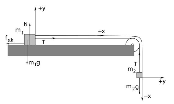
Suppose a block of mass  $m_1$  sits on a table. The coefficients of static and kinetic friction between the block and the table are  $\mu_s > \mu_k$  and  $\mu_k$  respectively. This block is attached by an "ideal" massless unstretchable string running over an "ideal" massless frictionless pulley to a block of mass  $m_2$  hanging off of the table. The blocks are released from rest at time t = 0.
