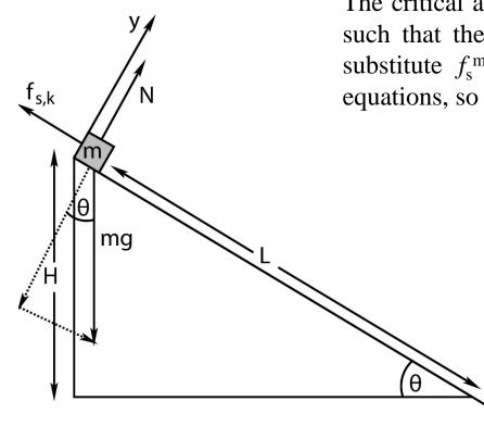
The critical angle is the angle where  $f_s$  is as large as it can be such that the block barely doesn't slide. To find it, we can substitute  $f_s^{\text{max}} = \mu_s N_c$  where  $N_c = mg \cos(\theta_c)$  into both equations, so that the first equation becomes:
