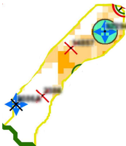
Figure 6. One of blocks of prediction map for site 1. Blue crosses mean injection wells, any color dots mean production wells, red and black crosses mean well was disabled. Brown color shows value of prediction - the darker the higher
