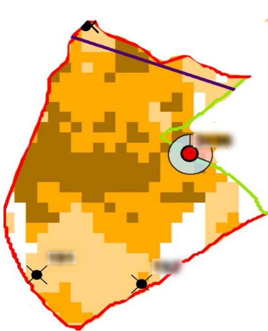
Figure 7. One of blocks of prediction map for site 2. Blue crosses mean injection wells, any color dots mean production wells, red and blacks crosses mean well was disabled. Brown color shows value of prediction - the darker the higher
