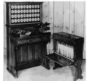
the first electrically driven device. It utilized punched cards and metal rods which passed through the holes to close an electrical circuit and thus cause a counter to advance. This machine was able to complete the calculation of the 1890 U.S. census in 6 weeks compared with 7 1/2 years for the 1880 census which was manually counted.
