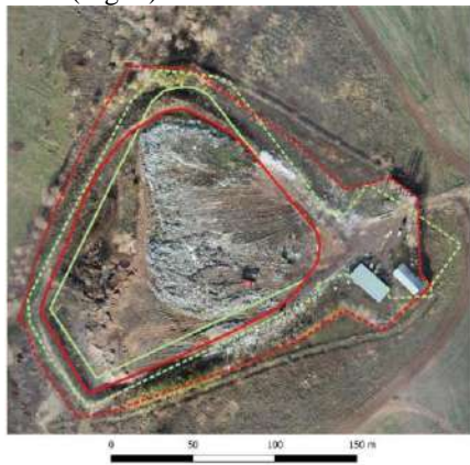
Figure 2: Orthophotomap of the landfill territory (solid green – the project boundaries, solid red - the actual contour of the storage area).
