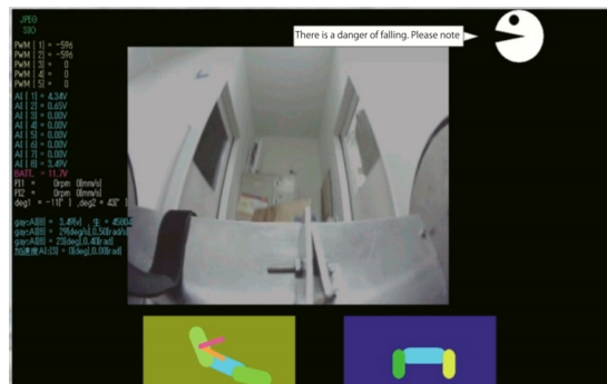
Fig. 1. Operator screen with support information from "Scott 1" [11].
