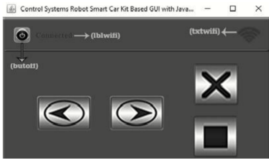
Fig. 2. GUI for operator of 4WD Smart Car Robot [10].
