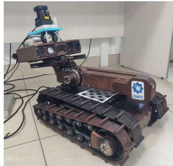
Fig. 4. Servosila Engineer crawler-type mobile robot.
