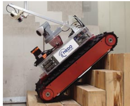
Figure 16. Going down through CBL OO1 posture at \theta_{CPQ} = 87.5 deg, using a tricky horizontal barrier.
