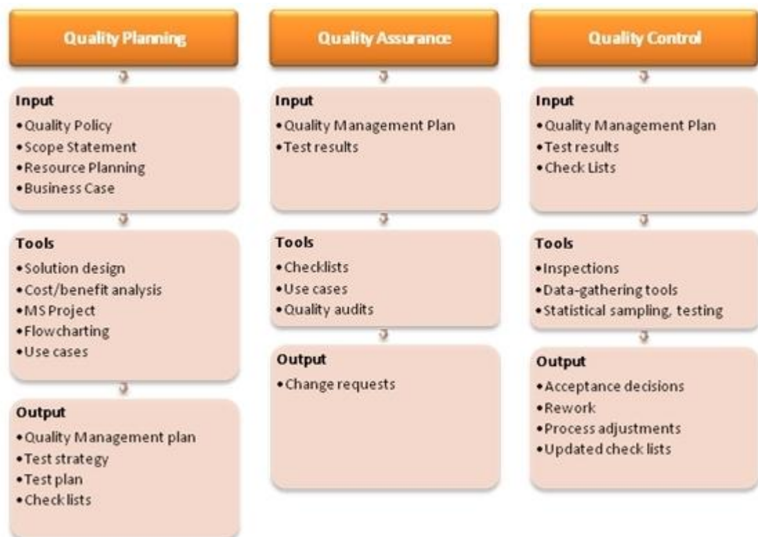
Fig.1 The structure of the project quality management
