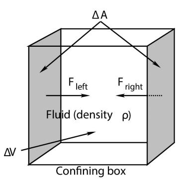
In figure we see a box of a fluid that is confined within the box by the rigid walls of the box.
