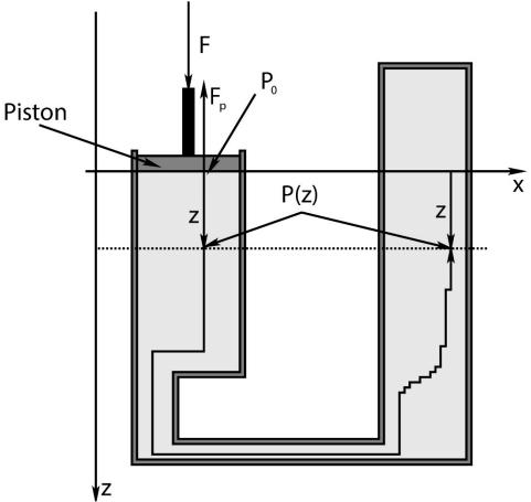
Now consider the following. Suppose we start with pressure  $P_0$  (so that the pressure at these two points is P(z), but then change *F* to make the pressure  $P'_0$  and the pressure at the two points P'(z). Then:
