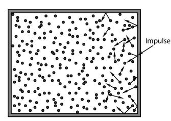
Many particles all of mass *m* are *constantly moving* in random, constantly changing directions (as the particles collide with each other and the walls) with an average kinetic energy related to the temperature of the fluid. Some of the particles (which might be atoms such as helium or neon or molecules such as  $H_2$  or  $O_2$ ) happen to be close to the walls of the container and moving in the right direction to bounce (elastically) off of those walls.
