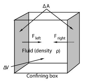
A fluid in static equilibrium has the property that every single tiny chunk of volume in the fluid has to *independently* be in force *equilibrium* – the total force acting on the differential volume chunk must be *zero*.
