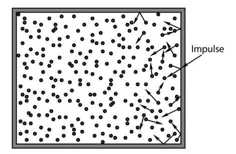
A large number of atoms or molecules are confined within in a "box", where they bounce around off of each other and the walls. They exert a *force* on the walls equal and opposite the force the walls exert on them as the collisions more or less elastically reverse the particles' momenta perpendicular to the walls.
