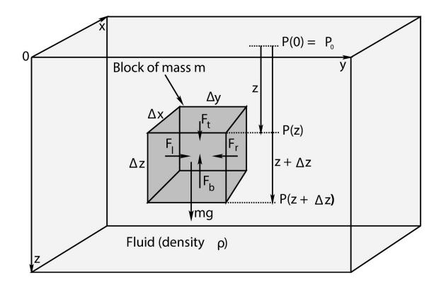
A solid chunk of "stuff" of mass m and the dimensions shown is immersed in a fluid of density  $\rho$  at a depth z. The vertical pressure difference in the fluid (that arises as the fluid itself becomes static static) exerts a vertical force on the cube.
