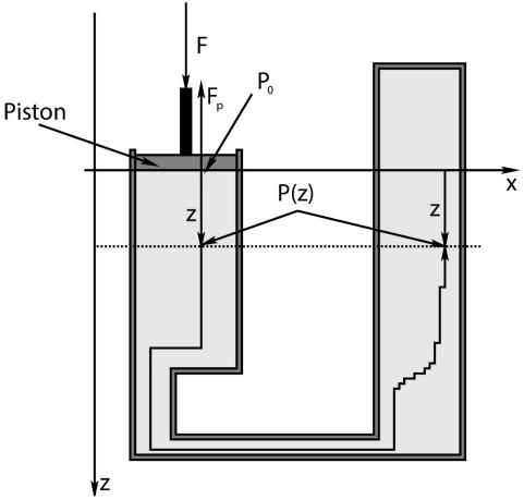
We can push down (or pull back) on the piston with any total downward force F that we like that leaves the system in equilibrium. Since the piston itself is in static equilibrium, the force we push with must be opposed by the pressure in the fluid, which exerts an equal and opposite upwards force:
