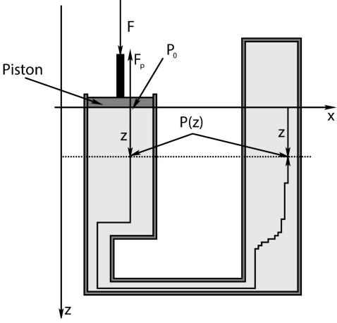
Suppose, that we have an *incompressible fluid* e.g. water confined within a sealed container by e.g. a *piston* that can be pushed or pulled on to *increase or decrease* the *confinement pressure* on the surface of the piston.
