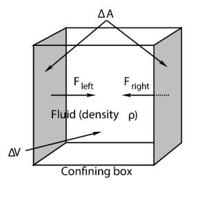
We can now make a few very simple observations about the forces exerted by the walls of the container on the fluid within. First of all the mass of the fluid in the box above is clearly:
