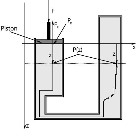
The pressure at a depth z in the container is then
