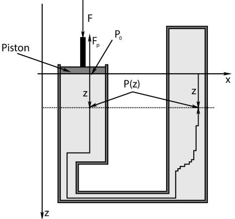
We recall that the pressure changes only when we change our depth. Moving laterally does not change the pressure, because e.g. dP/dx = dP/dy = 0. We can always find a path consisting of vertical and lateral displacements from z = 0 to any other point in the container – two such points at the same depth z are shown in figure, along with a vertical/horizontal path connecting them. Clearly these two points *must have the same pressure* P(z)!
