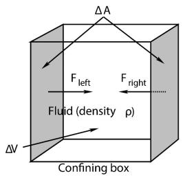
From this simple argument we can conclude that the average force exerted by any wall is proportional to the area of the wall. This force is therefore most naturally expressible in terms of pressure:
