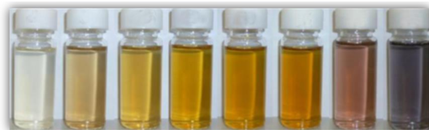
Figure 2. Nanoparticles of various shape and size in solution – the plasmon resonance determines the color.
