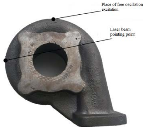
Fig 11. The body of TC turbine with the laser sensor beam guidance point and the place of free oscillation excitation
