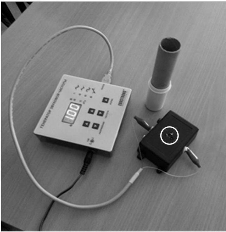
Figure 2. The appearance of the device. The diodes of three colors are marked with a white circle (model groups of three cones).
