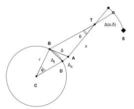
**Fig. A.1.** Error in parallax reduction due to uncertainties in the position of observer. In the case of a small angle  $\phi$ , one can use  $\Delta^2 = \Delta_1^2 + \Delta_h^2$ .
