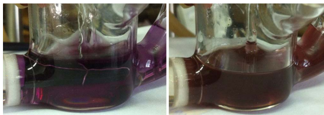
Figure 4. Pictures of 1.3 mM C_{60} + 1.0 mM AuCl solution in DCB-DMF (2:1)/0.1 M Bu_4NCl medium before (left) and after (right) the electrolysis at -0.4 V ( Q = 1.0 F with respect to AuCl).
