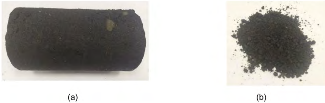
Figure 5—(a) Initial full size core, (b) grinded core (grain size 0.1 \div 1 mm).
