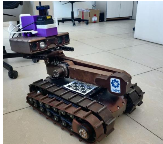
Figure 2. Servosila engineer robot, courtesy of Servosila company.
