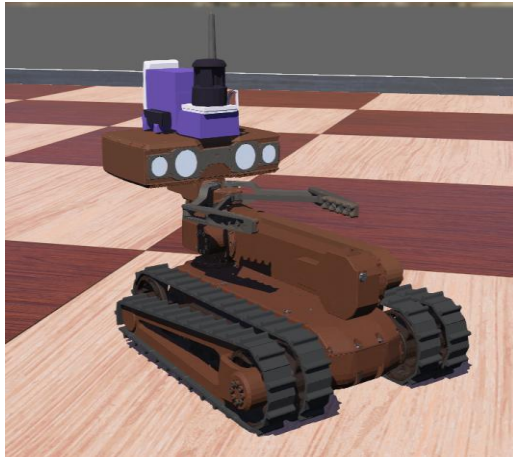
Figure 3. Simulation model of Servosila Engineer in Webots simulator.
