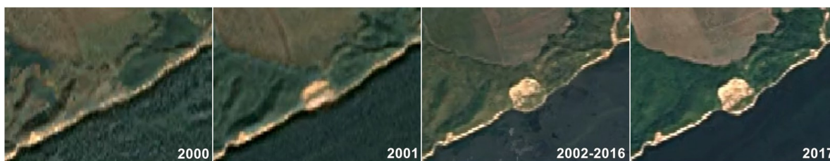
Figure 2. Landslide II development in the 2000-2017 period (Google Earth Timelapse).
