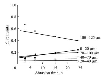
**Fig. 2.** Concentration of different KDI catalyst fractions versus abrasion time in our experiment with initial fraction 1 (points) and in calculations (lines).
