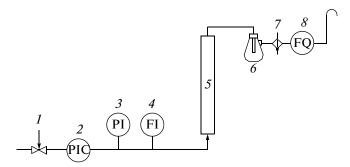
**Fig. 1.** Schematic of the unit for estimating the mechanical strength of catalysts in an air jet: (1) valve, (2) SDV-6 pressure stabilizer, (3) manometer, (4) rotameter, (5) abrasion vessel, (6) coarse filter, (7) fine filter, (8) gas counter.
