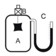
vessel A and the valve B is closed immediately after that, the pressure and temperature in the vessel will increase. Since there is a heat flow through the walls of the vessel, the temperature inside the vessel will become equal to the ambient (room) temperature in a while, and the pressure will decrease somewhat to a new value
