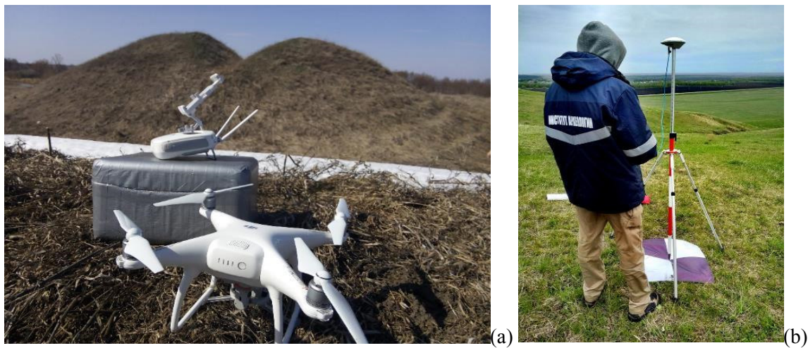
Figure 1. Quadcopter DJI Phantom 4 (a), special mark georeferencing by GNSS receiver (b).
