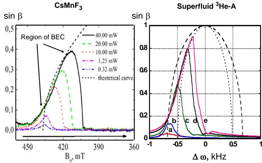
**Figure 1.** On a left side the amplitude of CW NMR signal from CsMnF<sub>3</sub> as a function of external magnetic field for different energy of excitation. The dashed line is a theoretical curve follows the equations (6,7). On the right side shown the similar results measured in <sup>3</sup>He-A in aerogel
