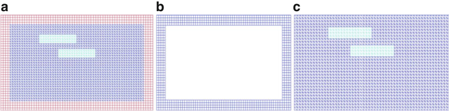
Fig. 1 (a) Geometry of the hybrid mesh. This is a combination of the quadrilateral mesh in the subdomain \Omega_{FDM} (b), where we apply FDM, and the finite element mesh in the inner domain \Omega_{FEM} (c), where we use FEM. The solution of the inverse problem is computed in \Omega_{FEM} . The trace of the solution of the forward problem (66) is recorded at the top boundary \Gamma_1 of the finite element domain \Omega_{FEM}
