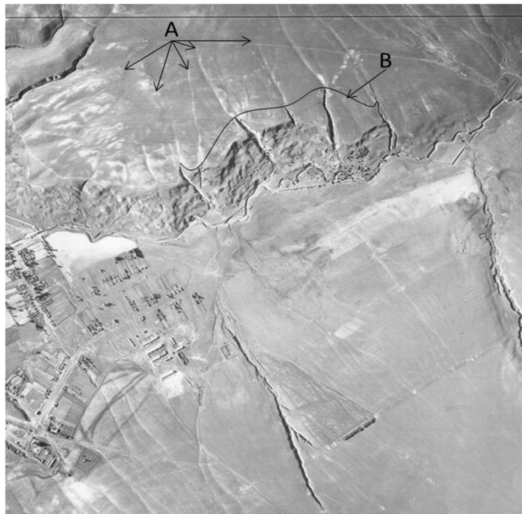
Figure 1. The allocation of erosion belts using interpretation aerial photographs. A is the detection of the lower boundary of the sheet and rill erosion at the tops of stream erosion; B is the boundary of the gully erosion belt changed by landslide processes (aerial photograph fragment; scale 1:17,000).
