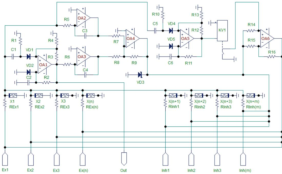
Figure 2. The wiring schematic of memristive artificial neuron
