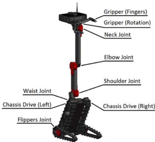
Fig. 1. Servosila Engineer servo drive scheme.
