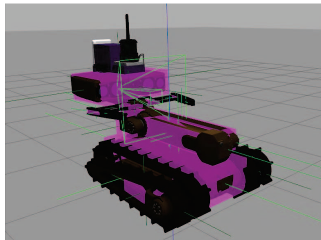
Fig. 8. Inertia of the model simulation model (inertial modules marked purple).
