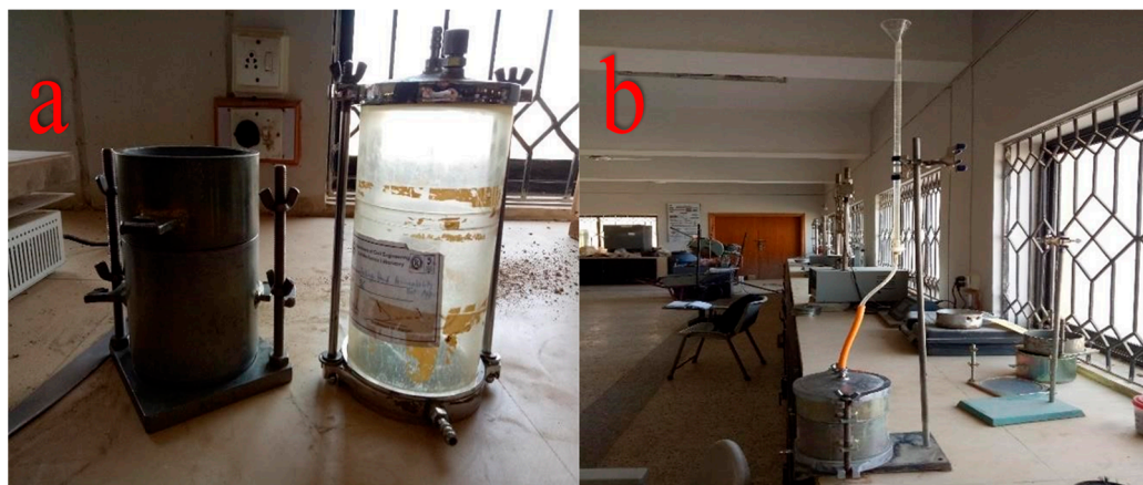
Figure 1. (a) Permeability apparatus and (b) modified permeability apparatus.
