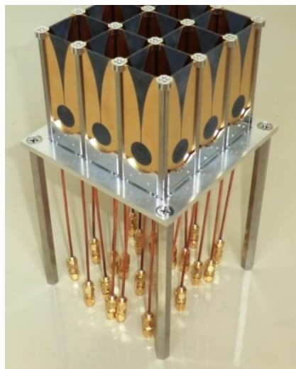
Figure 10.4. Vivaldi antenna with 24 elements (Kikuch et al., 2014)
