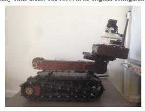
Fig. 1. Servosila Engineer crawler-type robot with a Hokuyo UTM-30LX-EW LRF mounted on its top.
