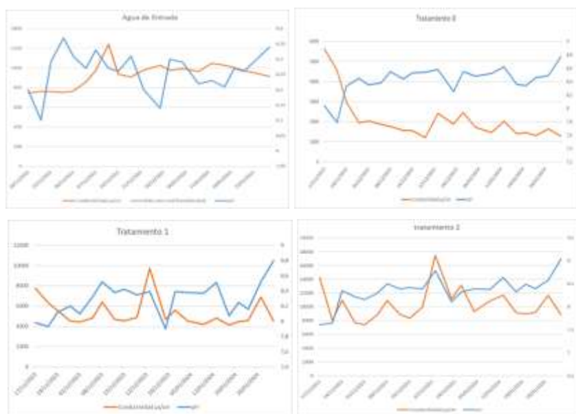
Figure 1. Behaviour of pH, conductivity in the inlet and outlet water (Treatment 0, Treatment 1, Treatment 2) during the experiment.
