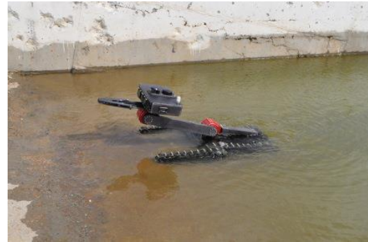
Fig. 2. Servosila Engineer crawler rescue robot (photo by courtesy of “Servosila” company).
