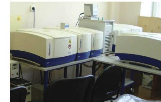
Minispec MQ20 - instrument for investigation of magnetic properties of metal-containing polymeric materials
