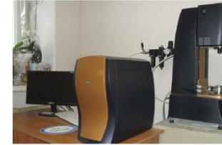
Rheometr DHR-2 used for development of new epoxy composites
