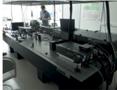
Femtosecond laser system, Coherent Inc., USA: it includes oscillator Mira-5 (wavelength 800 nm, pulse duration after compression less than 15 fsec), regenerative amplifier ELite USP (wavelength 800 nm, pulse duration 35 fsec, pulse energy 1.5 mJ), optical parametric amplifiers OPeRa Solo
