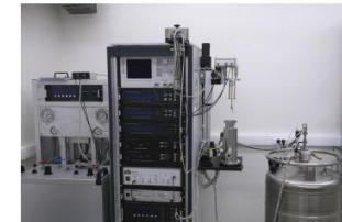
Dielectric spectrometer Novocontrol BDS Concept 80 (Germany) allows to measure the parameters of new functional composite materials in the wide frequency range 0.003 MHz - 3 GHz, at various external pressures 0-3000 MPa and temperatures -160 °C - +400 °C
