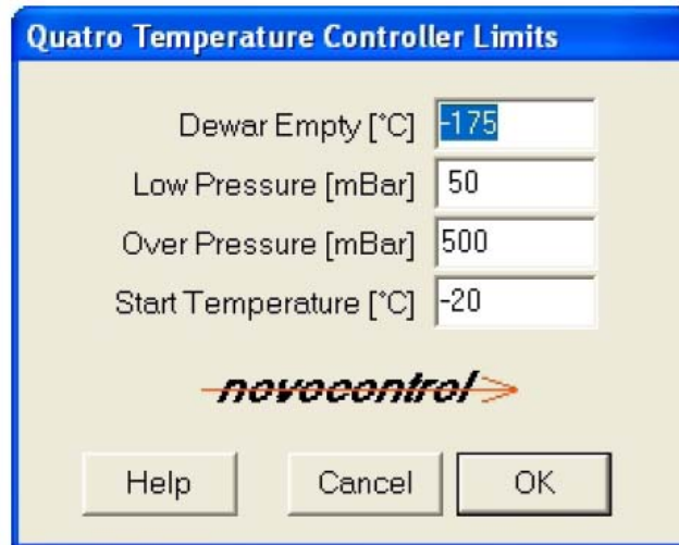
Figure 13. Sets the Quatro temperature controller safety limits.
